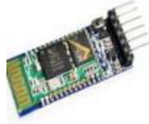
Figure 5: HC-05 Bluetooth Module
